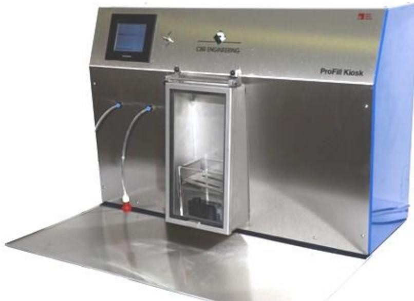
Now the built-in fluid sensors allow a high precision metering of ink. The accuracy of each independent line is reaching 0.1 ml! No other equipment supplies this precision in ink dosing! For refilling low ink volume cartridges this becomes necessary.
